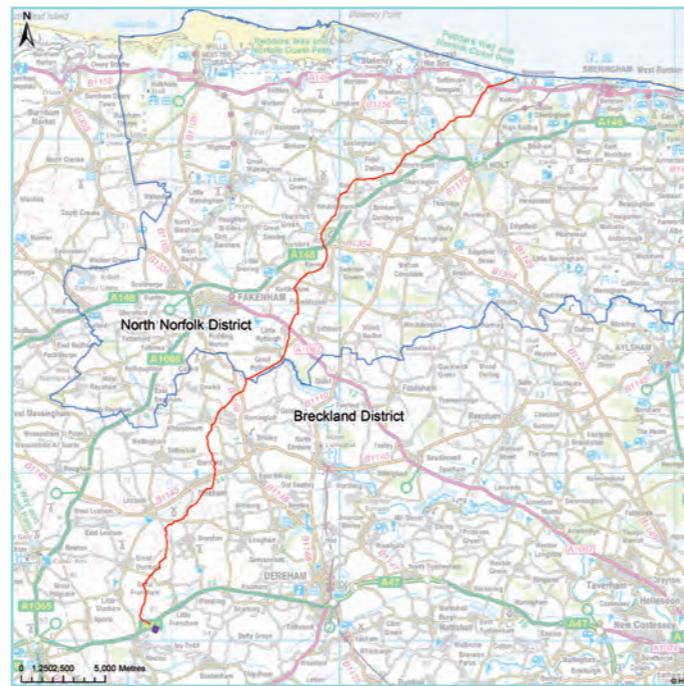
▶ The onshore cable route across Norfolk
